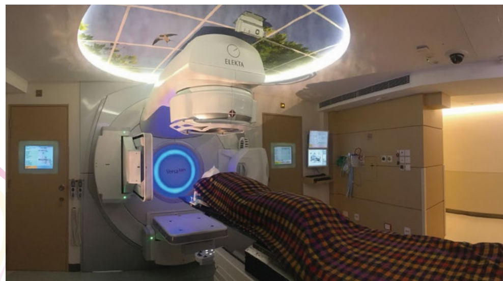
Versa HD™, the latest linear accelerator model, provides high precision radiation therapy that combines advanced image guidance, a multi-leaf collimating system, high dose rate, and a 6D couch to more effectively treat a wide range of cancers. Versa HD™ 直線加速器結合嶄新的影像導引技術、多葉式準直儀、高放射劑率及6D定位治療床，更有效治療各類腫瘤。
